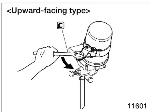
With an upward-facing oil filter, loosen drain plug 1 and air plug 2 in that order, then drain the oil out of filter 3.
