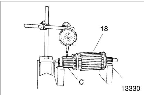
**(3) Runout of commutator**
