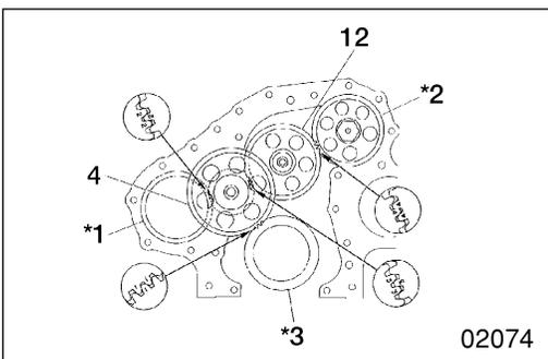
**4 12** Installing No. 1 and No. 2 idler gears
