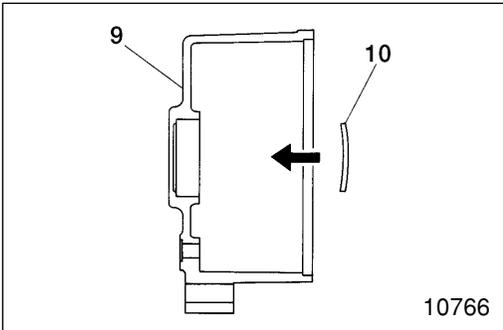
**10** Installation of conical washer
