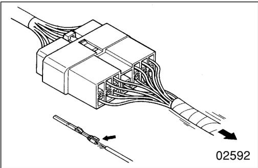
Check if harnesses are broken by pulling gently around the terminals.
