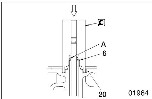
**6** Installing valve stem seals
