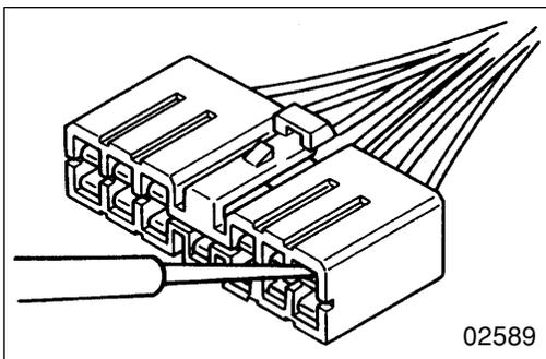
**Test with connectors disengaged**
