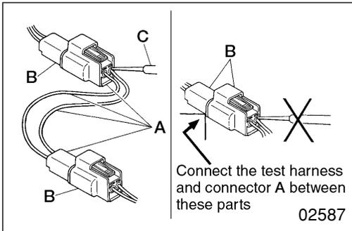
**Test with connectors engaged (continuity through circuit obtained)**
