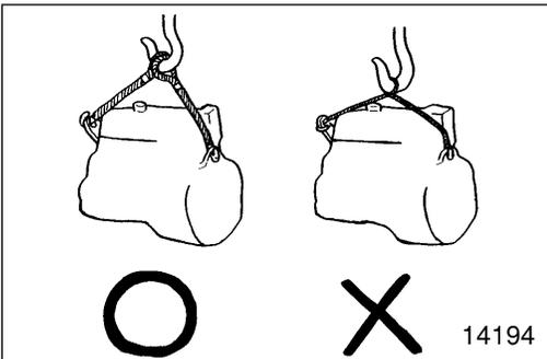
Pay special attention to safety when removing or installing heavy items such as engines, transmissions.
