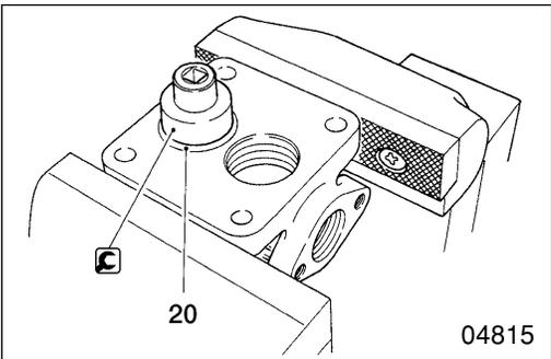
20 Removal and installation of delivery valve holder
