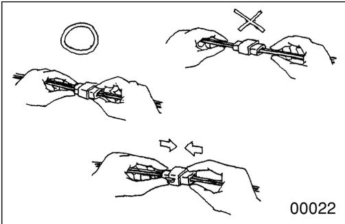
Pull the connector, and not the harness lead, to separate connectors. To separate a lock-type connector, first push toward arrow mark. To reconnect a lock-type connector, press the separated parts until they click together.
