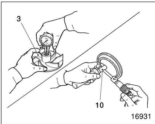
**3 10** Impeller-to-water pump shaft interference
