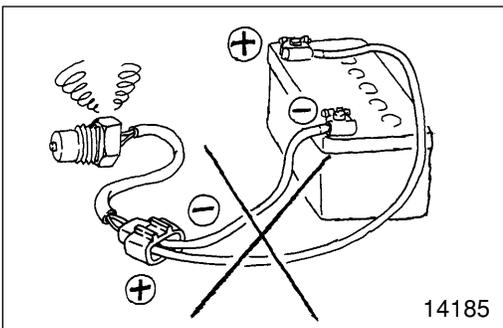
To apply voltage for testing, check that the positive and negative cables are connected properly, then increase voltage gradually from 0 volt. Do not apply voltage higher than the specified value.
