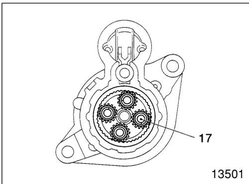
This starter uses planetary gear 17 in the reduction gear mechanism.
