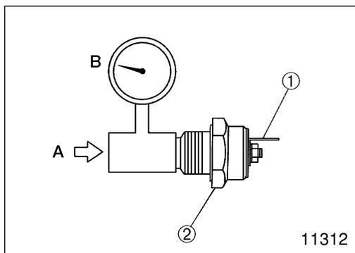
**Service procedure****3** Inspection of engine oil bypass alarm switch
