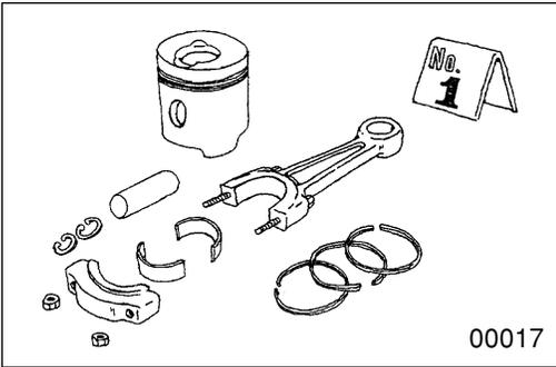
Put alignment marks on part combinations before disassembly and arrange the disassembled parts neatly. This will help avoid mismatching of the parts later.
