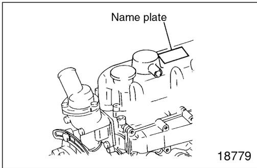
The name plate is attached to the portion shown in the illustration, and indicate the following items.
