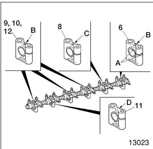
6 8 to 12 14 Installing rocker shaft brackets and rocker shaft
