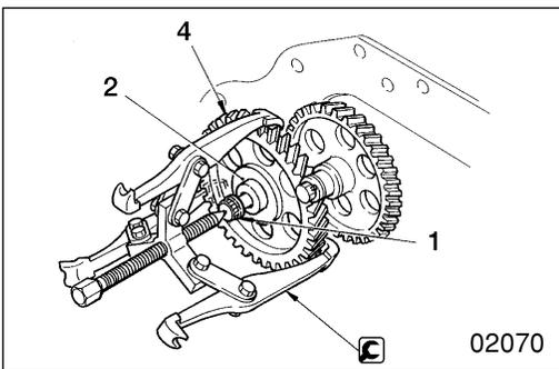
**2 4** Removing No. 1 idler shaft and No. 1 idler gear
