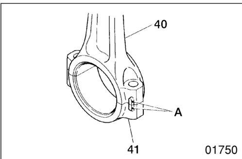
**40 41** Installation of connecting rod and connecting-rod cap
