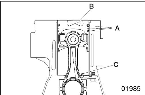
**5** Installing piston and connecting rod assembly
