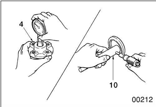
**4 10 Flange-to-water pump shaft interference**
