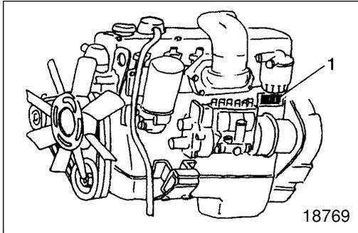
Engine number 1 is punch-marked on the left of the crankcase.
