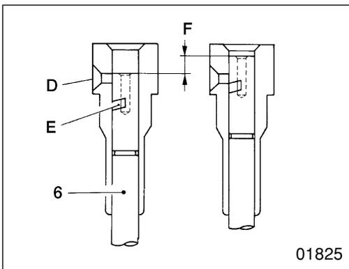
As the plunger 6 rises and its lead E meets the fuel inlet/outlet hole D, fuel flows through the center of the plunger and is expelled from the inlet/outlet hole. Regardless of how much further the plunger rises, no fuel feed takes place thereafter.
