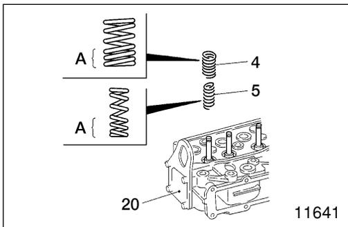
**4** **5** Installing outer and inner valve springs
