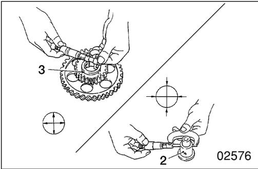
**2 3** No. 1 idler shaft and No. 1 idler gear bushing
