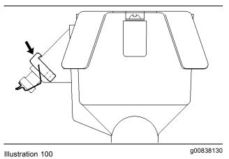
Retainer on the transformer's connector for the wiring harness
