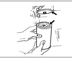
Illustration 64 Typical filter mounting base and gasket
